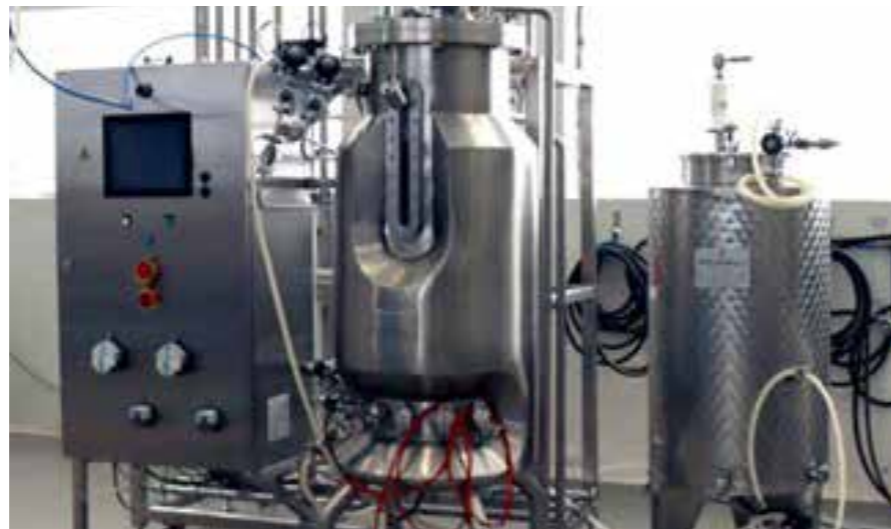
CNTA bioreactor in operation to produce biomass. Photo: CNTA
